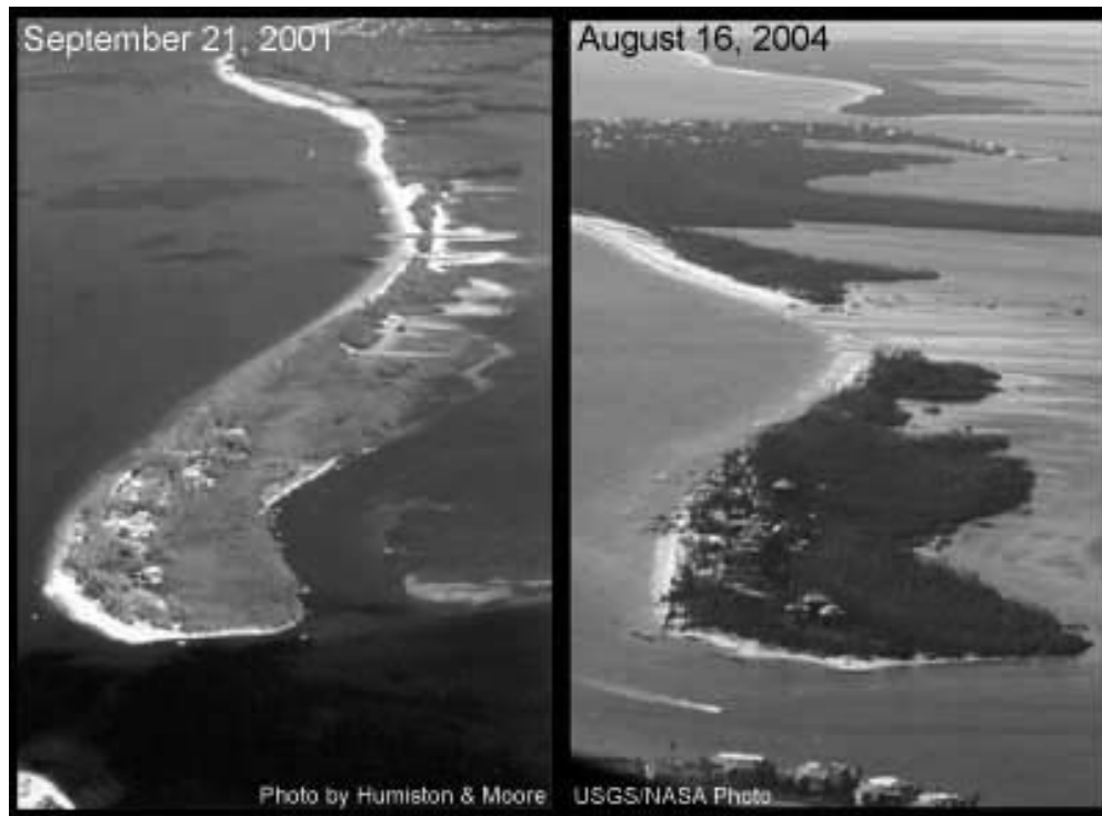
The pre-Hurricane Charley aerial photo on the left was taken several days following the passage of 2001's Tropical Storm Gabrielle. Note the two relatively small breaches in the central part of the island. On August 13, 2004, Hurricane Charley carved the 450-m-wide breach that is shown in the right photo. From U.S. Geological Survey.
