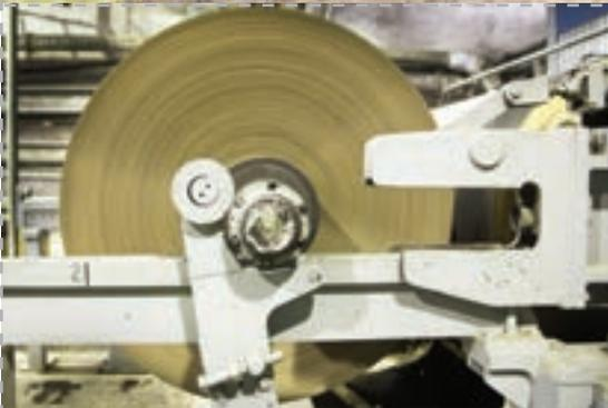
The sack-making machine folds and glues the sheets of paper.
