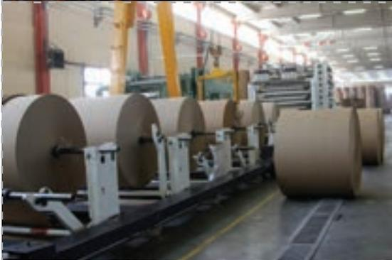
At the bag assembling plant, a sack-making machine cuts rolls of paper into sheets.
