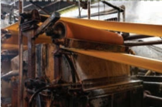
The pulp mixture moves through a series of rollers that press and dry it into rolls of paper.
