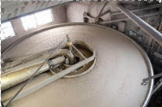
At the paper mill, 70% certified paper pulp, 15% noncertified paper pulp, and 15% recycled paper pulp are mixed together with water.
